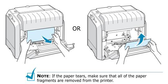
If you cannot find the jammed paper or there is any resistance removing the paper, go to step 3.
